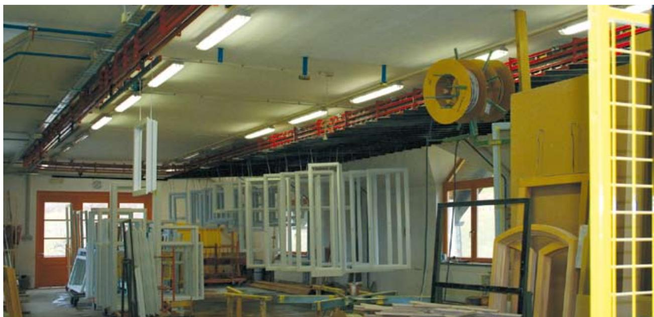
stalled an ultra-modern coating system (Finiture), with a 58 metre long conveyor (fig. 5), 65 piece-carrying bars that allow you to load up to 120 windows, and an anthropomorphic application robot (Cma Robotics) (fig. 6).
