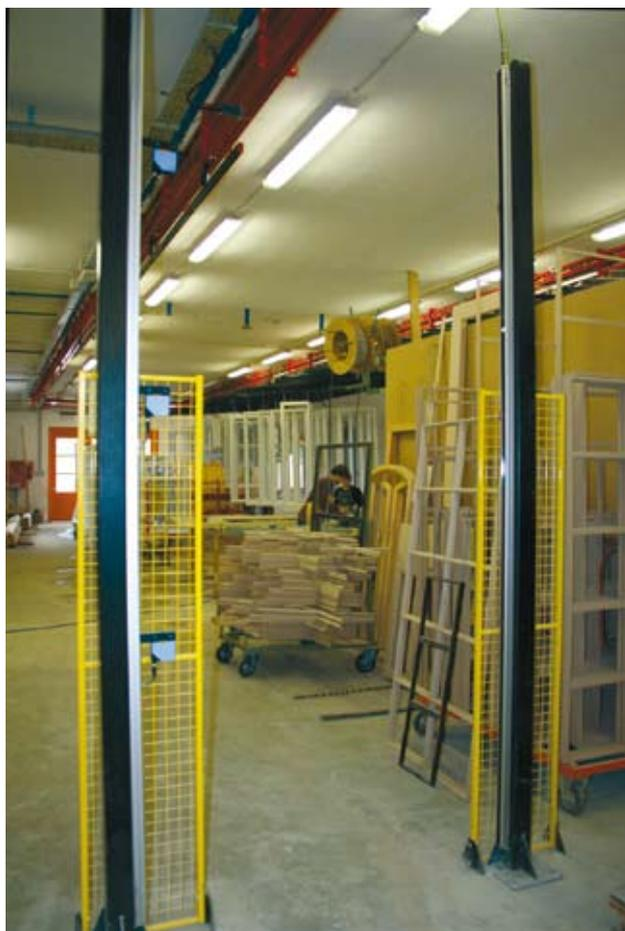
*7 – The scanner. On the left bar we can see the three sensors for assessing the dimensions.*
